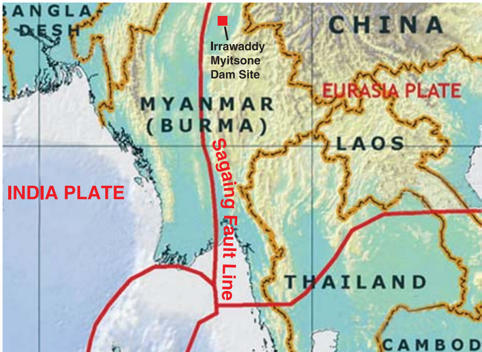
The Irrawaddy Myitsone Dam lies in an earthquake-prone area less than 100 kilometers from the Sagaing Fault Line where the India and Eurasia plates meet
